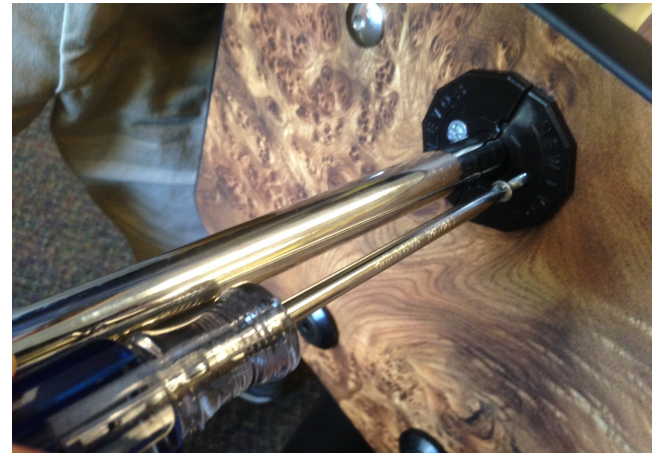
Screw the outer cabinet plates to the ones on the inside of the playing surface by lining-up the screw holes and cylinders on the other plates
