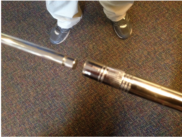
Insert the small diameter rod into the larger diameter rod
