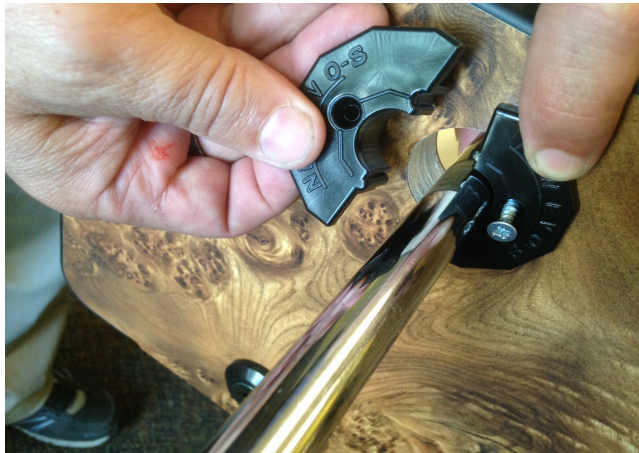
From the outer side of the game cabinet, place on each side of the rod, the positive and negative plates that DO have screw holes
