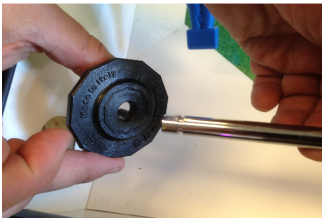
On the smaller rod at the other end, insert the full plate that has NO screw holes
